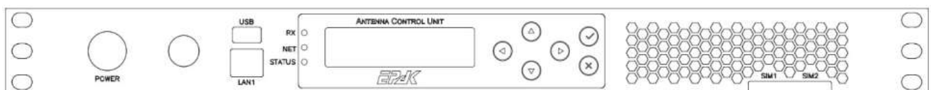
Figure 4.8: ACU Front view
