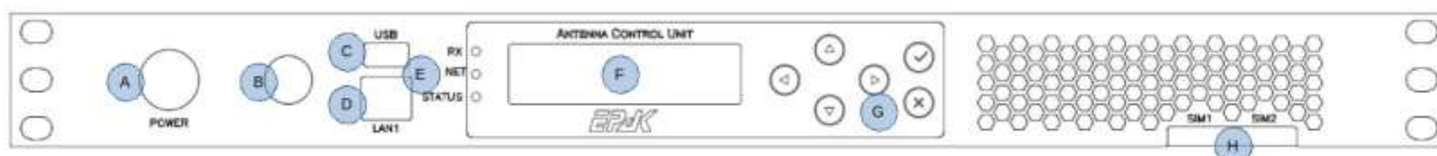
Figure 5.1: ACU Front view
