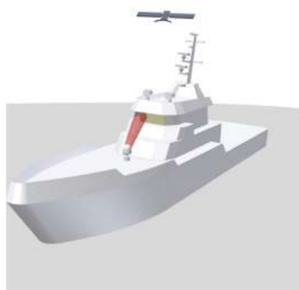
Bad location: in such a situation it is very likely to incur a wide blind spot.
