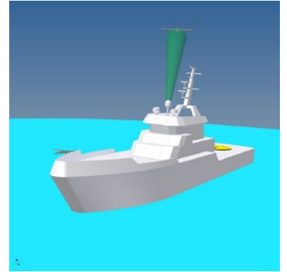
Best location: when possible, place the antenna on the top of the boat.
