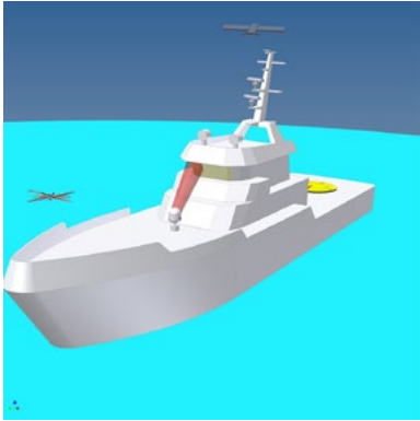
Bad location: in such a situation is very likely to incur a wide blind spot.
