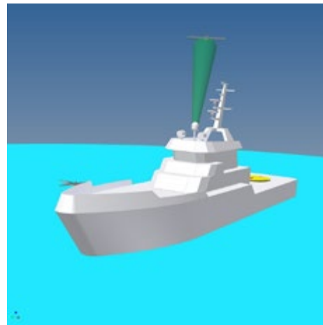
Best location: when possible, place the antenna on the top of the boat.
